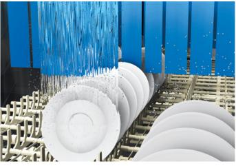
The final rinse function is only activated for sections of the belt that actually contain dishes.
