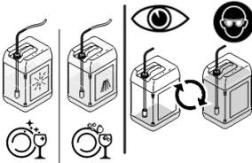
1. Remove the suction lance from the empty canister and insert it into a full canister.
