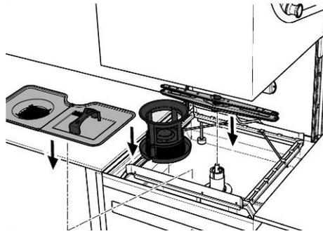
6. Insert filter, tank cover sieve and wash systems (top and bottom).
