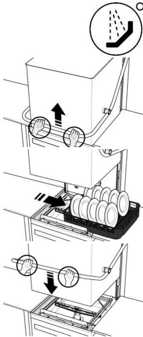
After the programme ends, the control light above the wash key turns off and an acoustic signal sounds.
