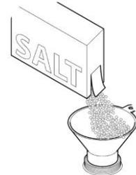
1. Open hood with both hands and fill salt solution container with 2.2 kg of regeneration salt (sodium chloride with a grain size of 0.3 - 1 mm). If possible, use a loading chute!
