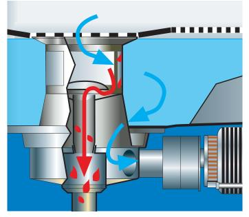
Outstanding cleaning results thanks to multiple filtration of tank water.
