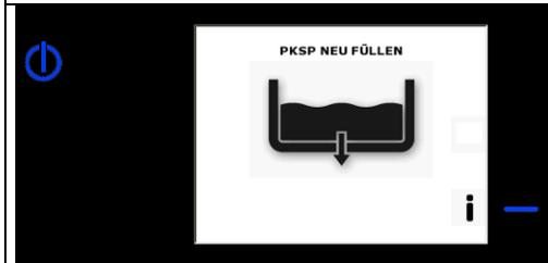
The pump rinse tank is drained and re-filled.
