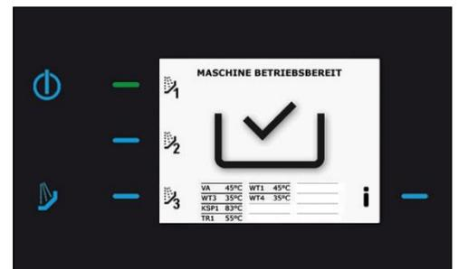
Once the wash tanks are filled and have been heated to the washing temperature, the display will show. Ready for operation
