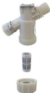
It is possible to clean the dirt screens without turning off the main water supply. The water supply is automatically cut off when the lower component in which the screen is located is unscrewed. This enables the screen can be easily cleaned during maintenance.
