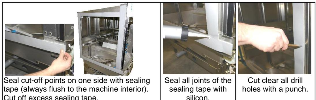
**Sealing a gap between two tanks:**
