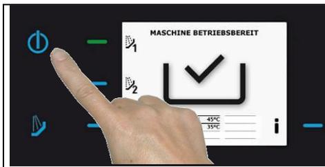
Press the "on-off" button to switch off the dishwasher.
