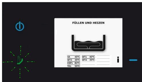
The green LED flashes. The wash tanks can be automatically filled and heated by means of the "Fill/Heat" button.
