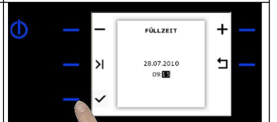
Enter the required date and time. Press the +/- button to change the value in the selected field. Then press >| to move to the next field. For example: 28.07.2010, 9:15 hrs
