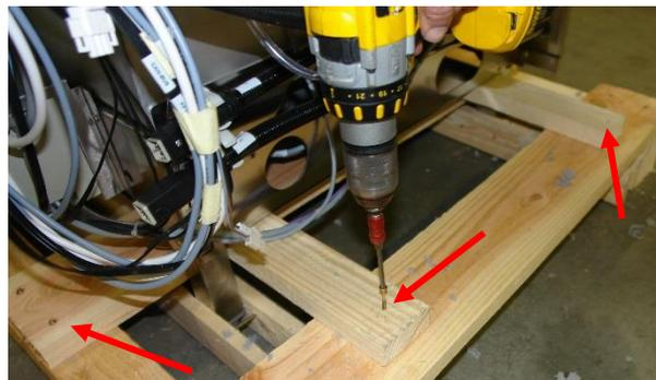
All the screws and bolts of the packing are now removed.
