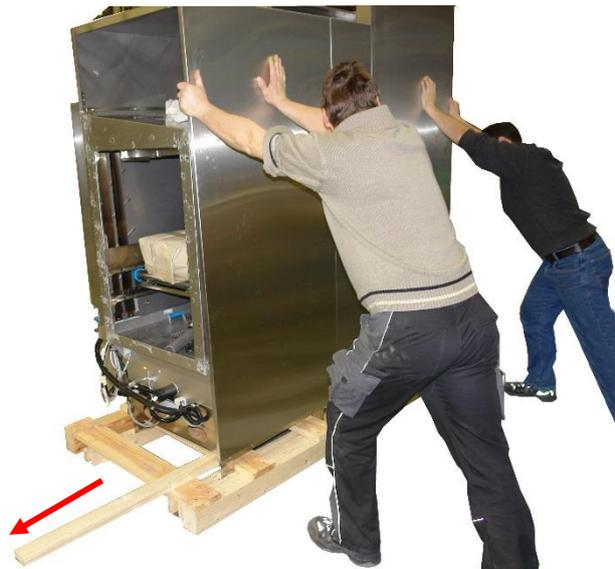
All the glands of the transport packaging are unbound, the machine will be lifted on one side and all the great longitudinal beams can now be pulled out without any effort under the machine.
