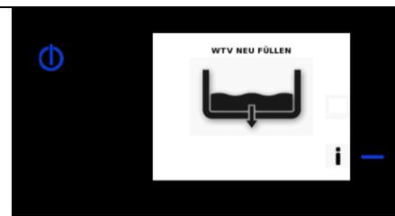
This drains the pre-clearing tank and refills all tanks.
