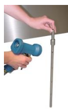
Clean the wash and rinse arms and their jets. Use a nylon brush to clean the jets. Check that the wash arms and end caps are complete and water-tight.
