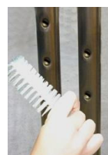
Clean the wash and rinse arms and their jets. Use a nylon brush to clean the jets. Check that the wash arms and end caps are complete and water-tight.
