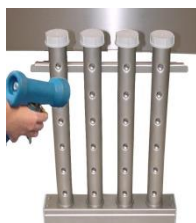
Clean the wash and rinse arms and their jets. Use a nylon brush to clean the jets. Check that the wash arms and end caps are complete and water-tight.
