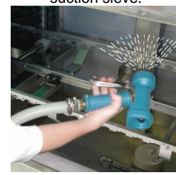
Clean the complete inner chamber of the tank with a hose.
