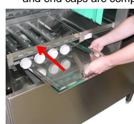
Clean the wash and rinse arms and their jets. Use a nylon brush to clean the jets. Check that the wash arms and end caps are complete and water-tight.
