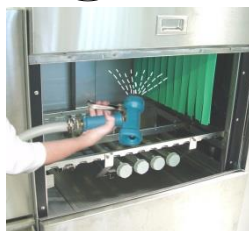
Spray the machine's internal chamber and the rear side of the vertical door with a hose
