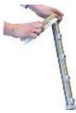
Clean the wash and rinse arms and their jets. Use a nylon brush to clean the jets. Check that the wash arms and end caps are complete and water-tight.
