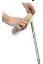
Clean the wash and rinse arms and their jets. Use a nylon brush to clean the jets. Check that the wash arms and end caps are complete and water-tight.
